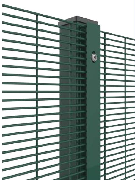
**358 security fence, also called anti-climbing, prison fence or high security fence, is a highly robust steel mesh fencing system. It consists of horizontal and vertical mesh wires that are placed close together to prevent people from putting their fingers through the holes and eventually climbing the fence.**
