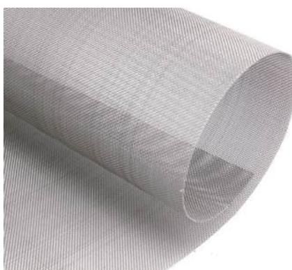
This wire mesh is made of 21% chromium, 2.5% molybdenum and 4.5% nitrogen nickel alloy. It has high strength, good impact toughness and good overall and partial stress corrosion resistance. In the world it known as 2205, trade mark is SAF2205.
