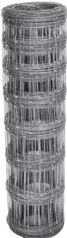
**Hinge knot field fence is the most common used type with economic benefits. Hinge joint is formed by wrapping the vertical wires around horizontal wires at each intersection. This spring shaped knot will provide the most elasticity to absorb the hardest impact energy as well spring back into its original shape. The hinged joint allows the necessary flexibility to move without breaking wires when pressure is placed on the fence by stock.**
