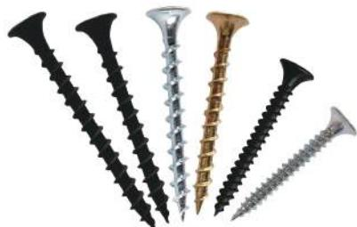
**Dry wall screws are divided into fine thread and coarse thread. The biggest difference between the two is that the former has double threads, which are suitable for the connection between gypsum board and metal keel with a thickness not exceeding 0.8mm, while the latter is suitable for the connection between gypsum board and wooden keel.**
