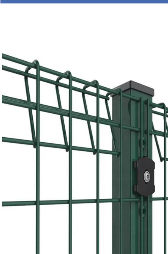
**Roll top fence, also known as BRC fence, features a unique and user-friendly closed and rolled beam section at the top and bottom edge of each panel, ensuring there are no sharp or raw edges. Typically constructed from heavy 5 mm wires, this design provides maximum rigidity and enhanced safety.**
